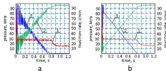
**Figure 1.** Dependences of pressure and flow rate in the acceleration mode of the mechatronic system: a – serial hydraulic motor; b – modernized hydraulic motor; 1 – pressure curve; 2 – curve of the flow of the working fluid through the hydraulic motor; 3 – curve of the flow of working fluid through the safety valve
