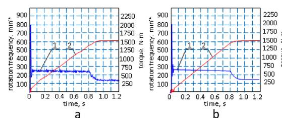
**Figure 2.** Dependences of changes in torque and frequency of rotation in the acceleration mode of the mechatronic system: a – serial hydraulic motor; b – modernized hydraulic motor; 1 – torque curve; 2 – curve of the frequency of rotation of the shaft of the hydraulic motor
